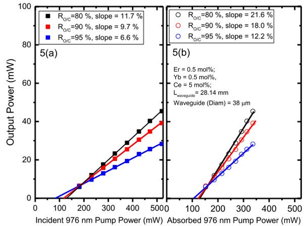
Fig. 5. Measured laser slope efficiencies of the 0.5 mol % Er<sup>3+</sup>:0.5 mol % Yb<sup>3+</sup>:5 mol % Ce<sup>3+</sup> doped ZBLAN chip,  $L=28.4$  mm. (a) as a fn. of incident 976 nm pump, and (b) as a fn. of absorbed 976 nm pump.
