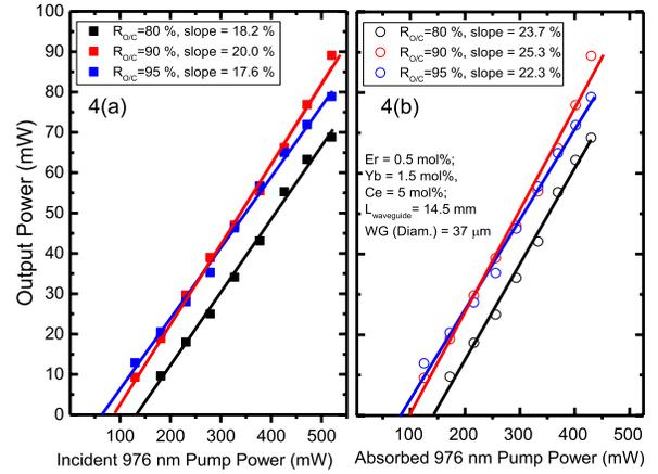
Fig. 4. Measured laser slope efficiencies of the 0.5 mol % Er<sup>3+</sup>:1.5 mol % Yb<sup>3+</sup>:5 mol % Ce<sup>3+</sup> doped ZBLAN chip laser,  $L=14.5$  mm. (a) fn. of incident 976 nm pump, and (b) fn. of absorbed 976 nm pump.
