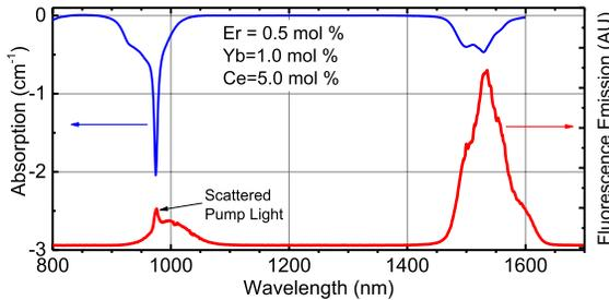
Fig. 2. Measured absorption in units of  $\text{cm}^{-1}$  of erbium ytterbium cerium doped ZBLAN (0.5 mol % erbium, 1.0 mol % ytterbium, 5.0 mol % cerium). The measured fluorescence emission spectrum for this composition is also shown.
