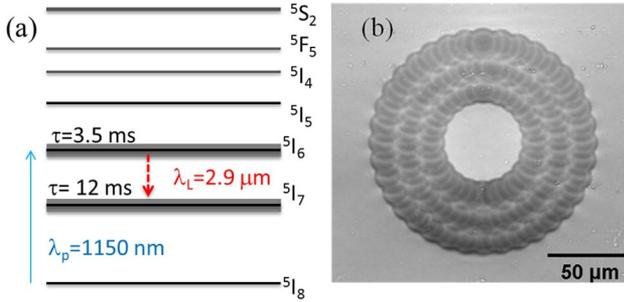
Fig. 1. (a) Energy level diagram of  $\text{Ho}^{3+}$  in ZBLAN glass. (b) End-on microscope image of the waveguide.
